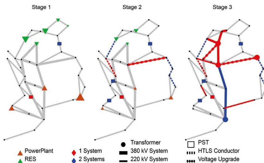
Figure: Required measures for maintaining system security
