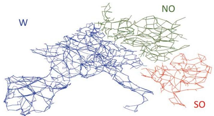
Figure: Representative Determined System Split in the European Interconnected Transmission Grid
