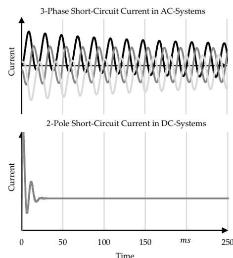
Figure: Schematic representation of short-circuit currents in AC and DC systems
