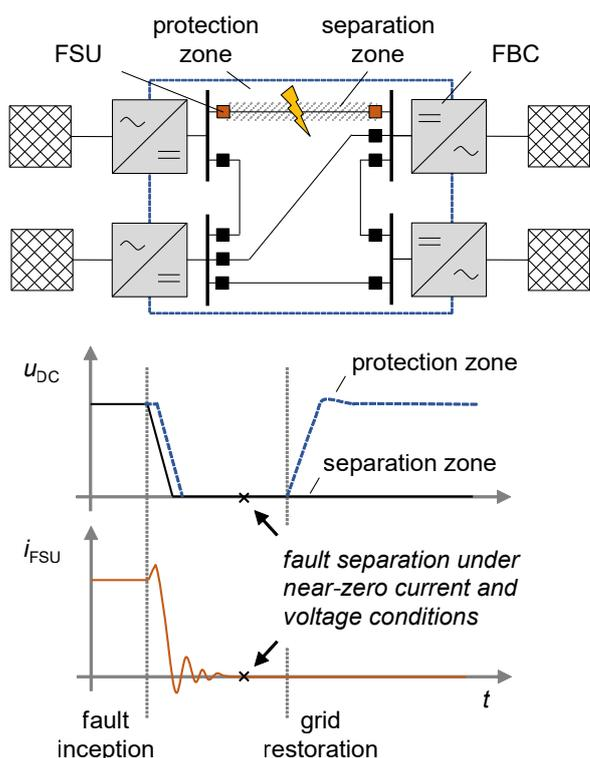
Figure: Schematic representation of the DC fault separation process in MTDC networks protected by FBCs
