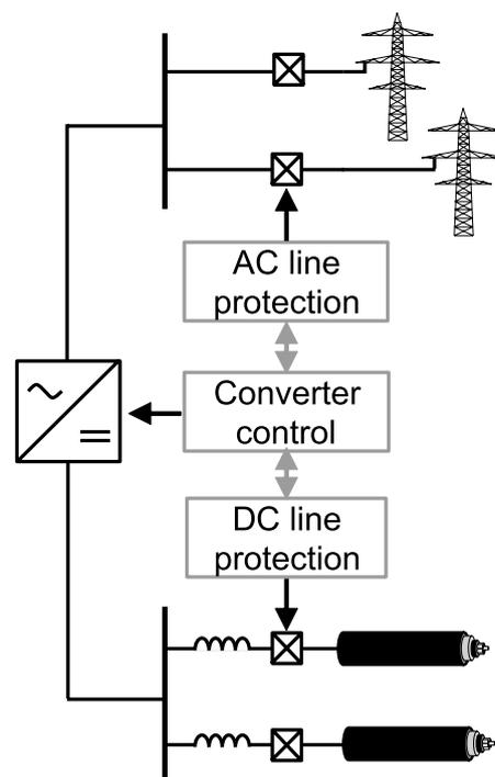
Figure: Protection and control system at the interface between AC and DC grids
