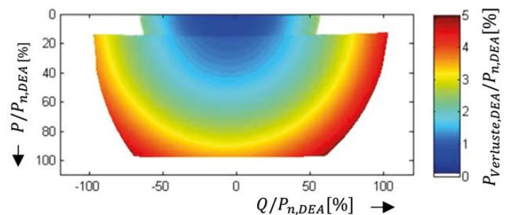
Figure: Model of internal losses of a representative wind park with doubly fed induction generators
