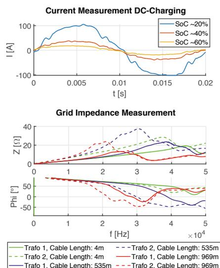
Figure: Current measurement of the charging process of an electric vehicle (top), grid impedance measurement for different grid characteristics (bottom)
