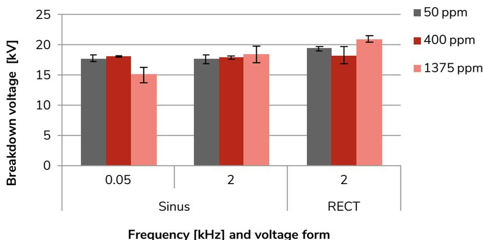
Figure: Breakdown voltage of MIDEI 7131 at water contents between 50 and 1375 ppm at 50 Hz and 2 kHz for sinusoidal and RECT voltages for homogeneous electric fields
