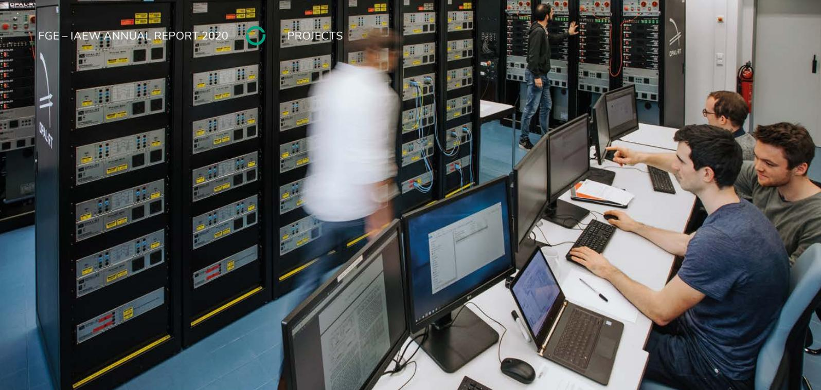
Figure: MMC Test Bench – Lab demonstrator for HVDC system investigations
