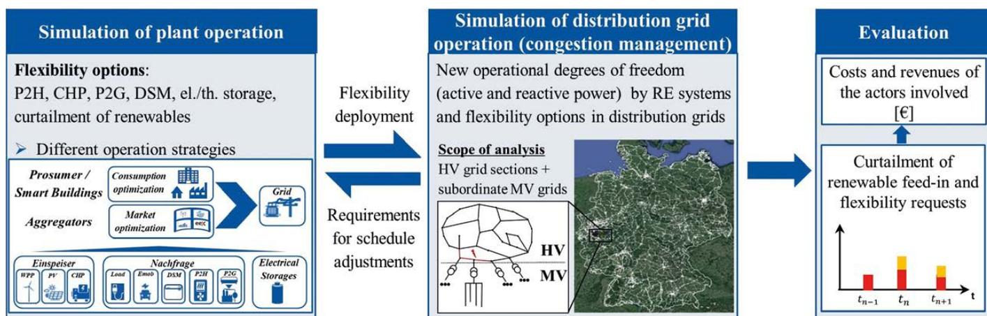
Figure: Schematic procedure of the simulation
