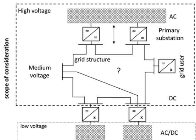
Figure: Medium voltage schematic network based on direct current technology
