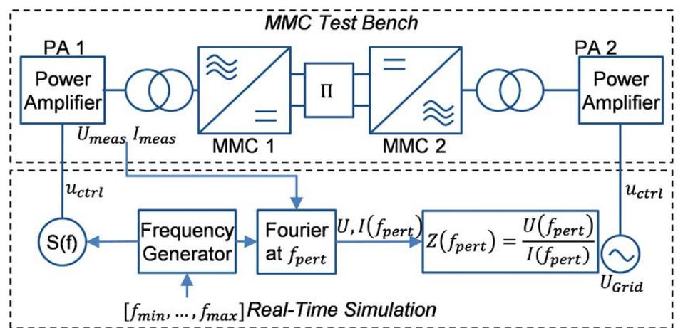
Figure: MMC Test Bench impedance measurement setup
