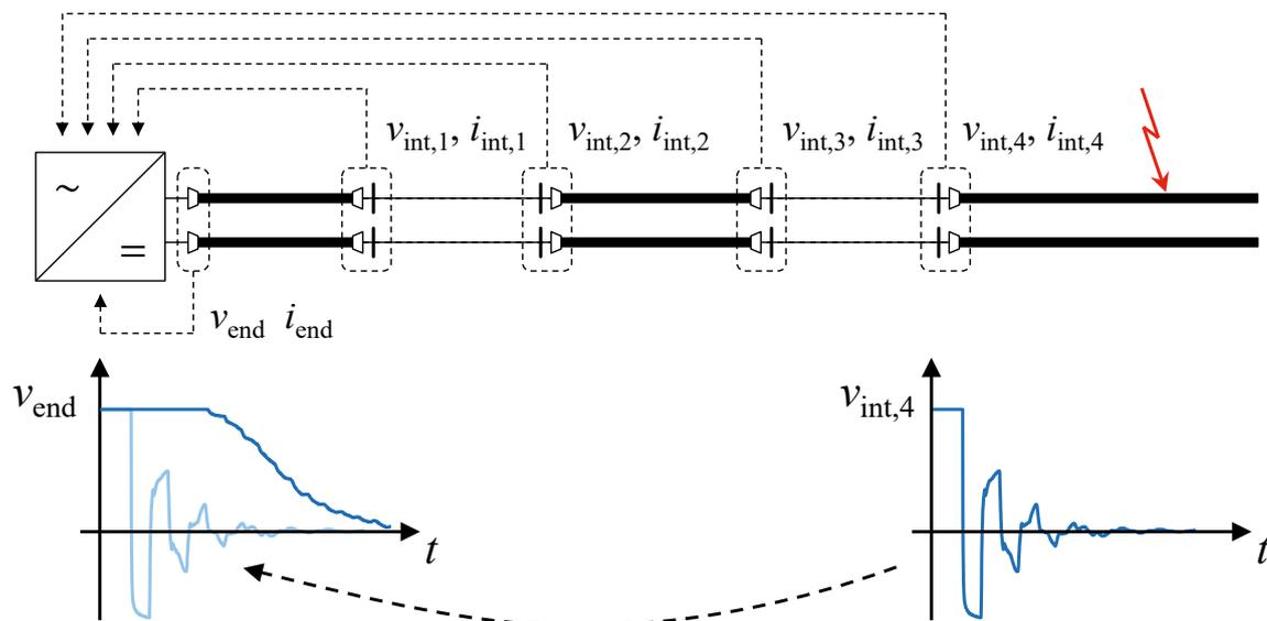
Figure: Protection of VSC-HVDC systems with mixed usage of power cables and overhead lines
