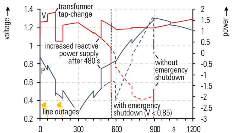
Figure: (In-)stable simulation results (voltage V and load P at load) during volatile supply task.
