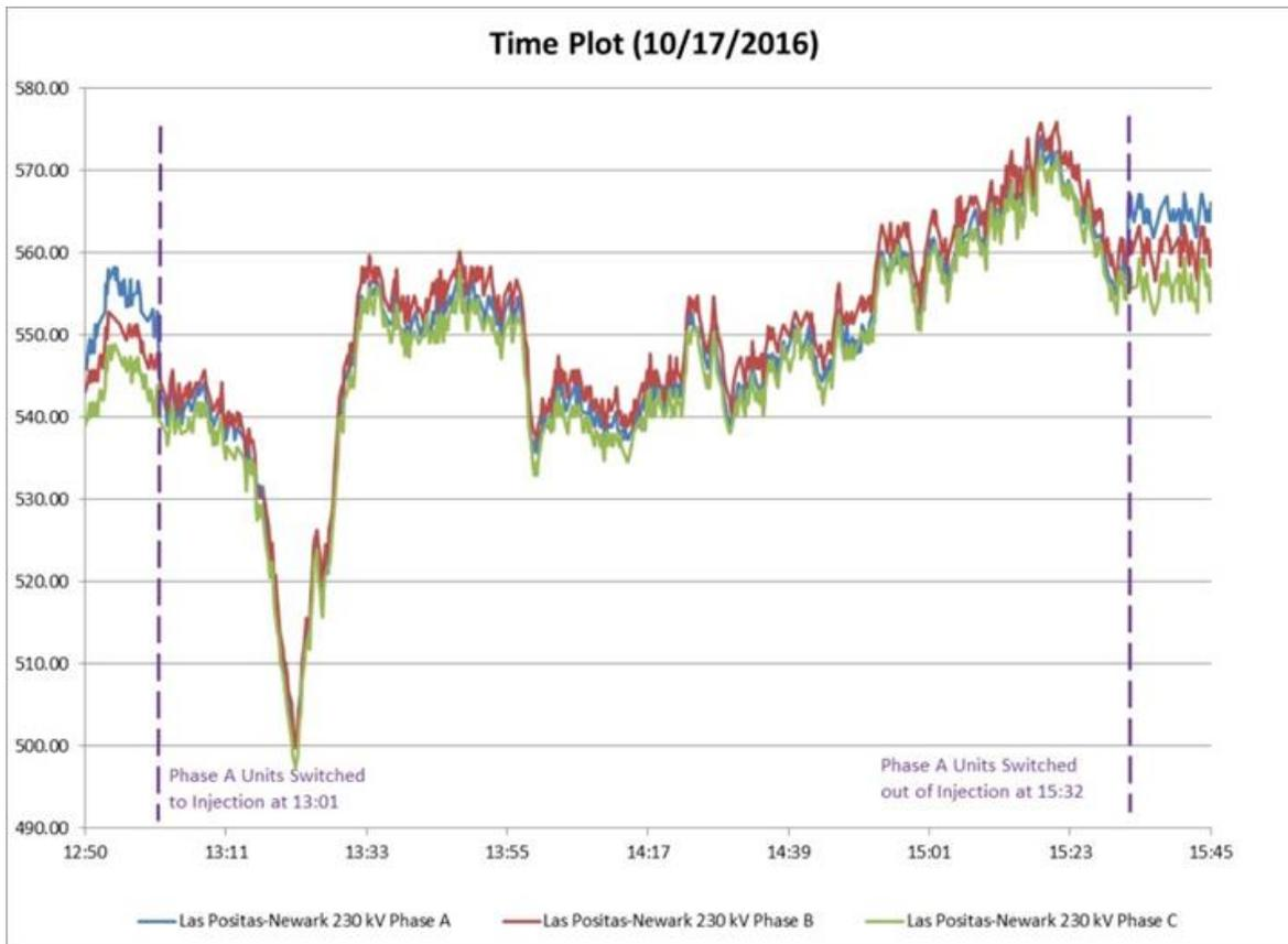
Figure 4-6 Phase Currents with DSRs on Phase A Only Injecting
