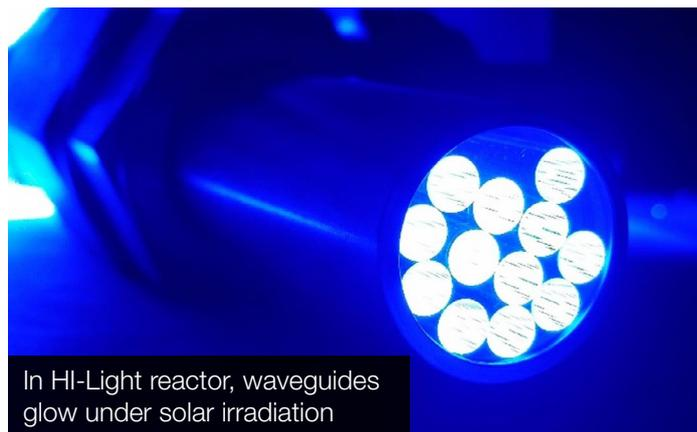
In HI-Light reactor, waveguides glow under solar irradiation
