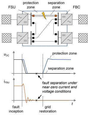
Figure: Schematic representation of the DC fault separation process in MTDC networks protected by FBCs
