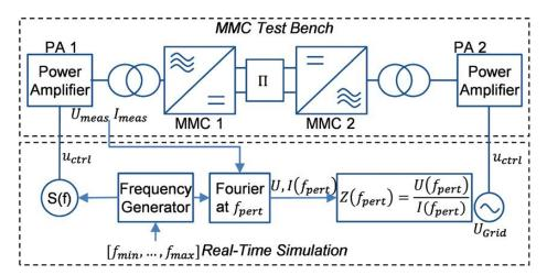
Figure: MMC Test Bench impedance measurement setup
