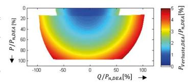
Figure: Model of internal losses of an representative wind park with doubly fed induction generators
