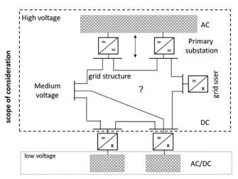
Figure: Medium voltage schematic network based on direct current technology
