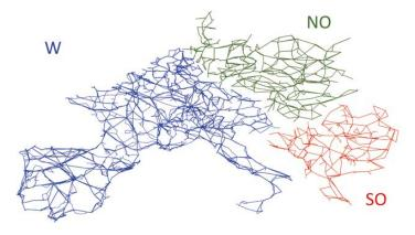
Figure: Representative Determined System Split in the European Interconnected Transmission Grid
