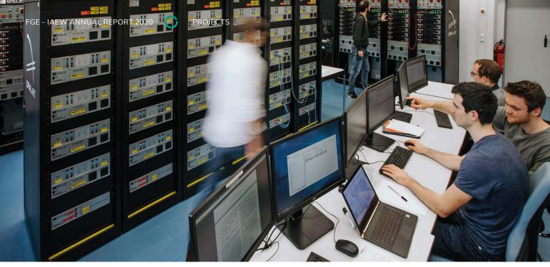
Figure: MMC Test Bench - Lab demonstrator for HVDC system investigations
