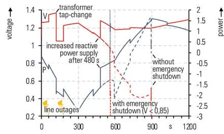
Figure: (In-)stable simulation results (voltage V and load P at load) during volatile supply task.
