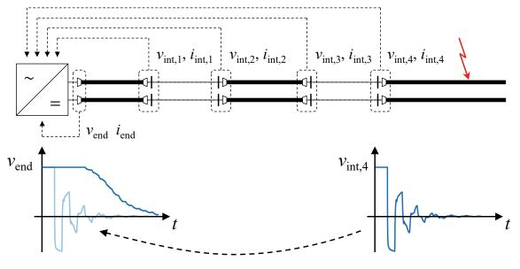
Figure: Protection of VSC-HVDC systems with mixed usage of power cables and overhead lines
