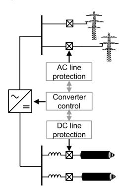
Figure: Protection and control system at the interface betwen AC and DC grids
