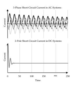
Figure: Schematic representation of short-circuit currents in AC and DC systems
