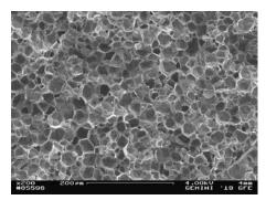
Figure: SEM image of the dry syntactic foam
