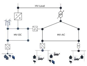
Figure: Schematical distribution grid with DC-application
