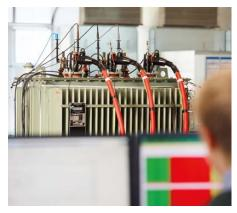
Figure: Acceleration measurements on a 400 kVA local network transformer in an open circuit test
